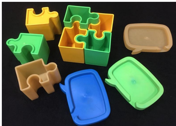
Fig. 1. Injection-molded prototypes of polyethylene/natural rubber blends
