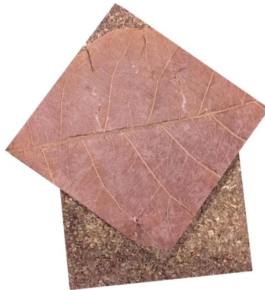
Fig. 1. Teak leaves sound insulation material for interior walls.
